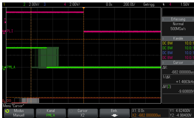
Fig. 7: Driving the load input of a PLI and a PMLA device without delay (long-term oscillogram with persistence)
