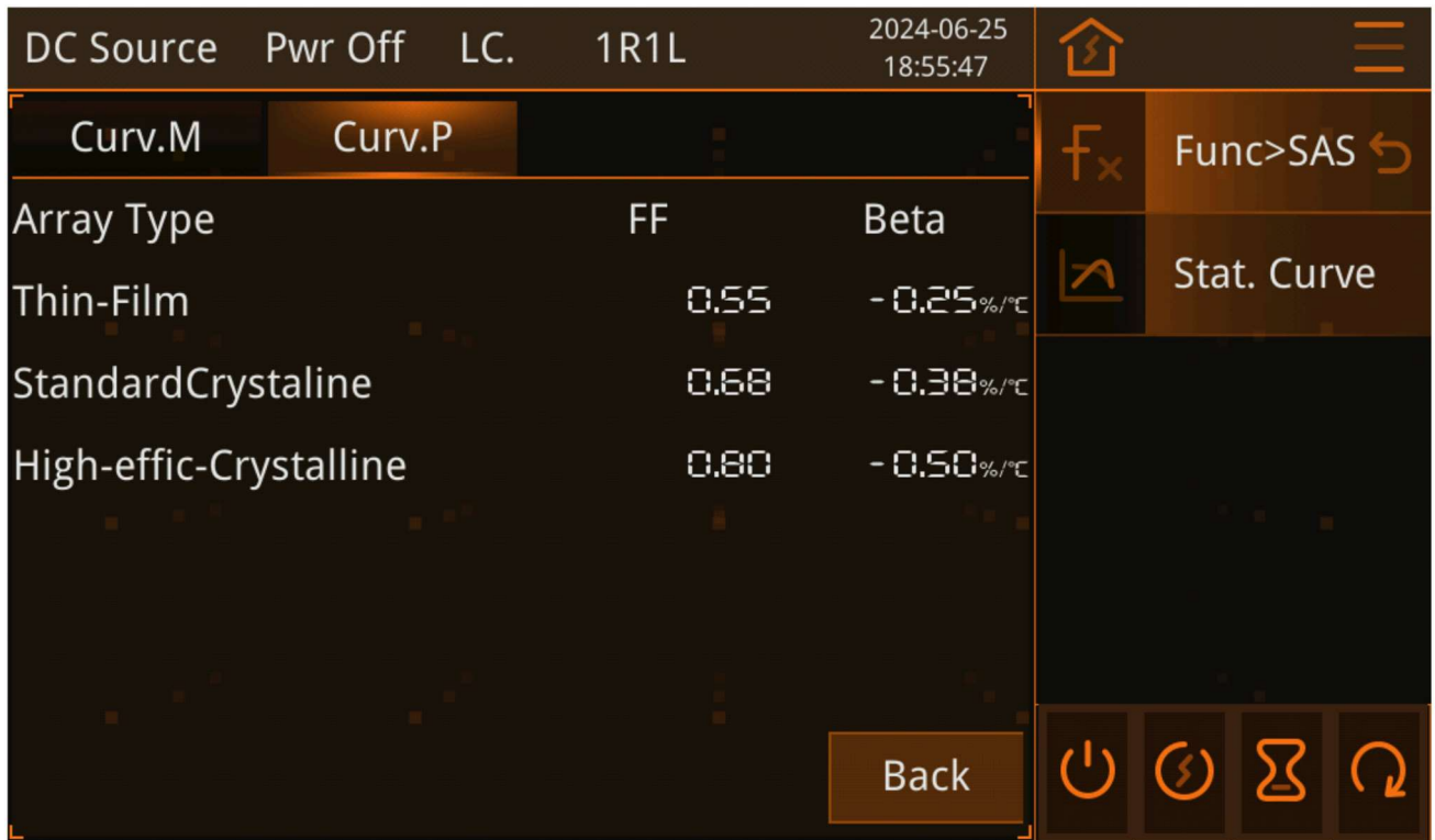
Figure 4-30: Curve Parameters (Sandia Advanced PV Tech) Interface
