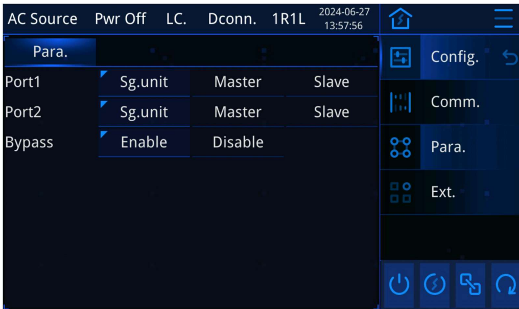
Figure 5-53 Parallel Operation Configuration Interface
