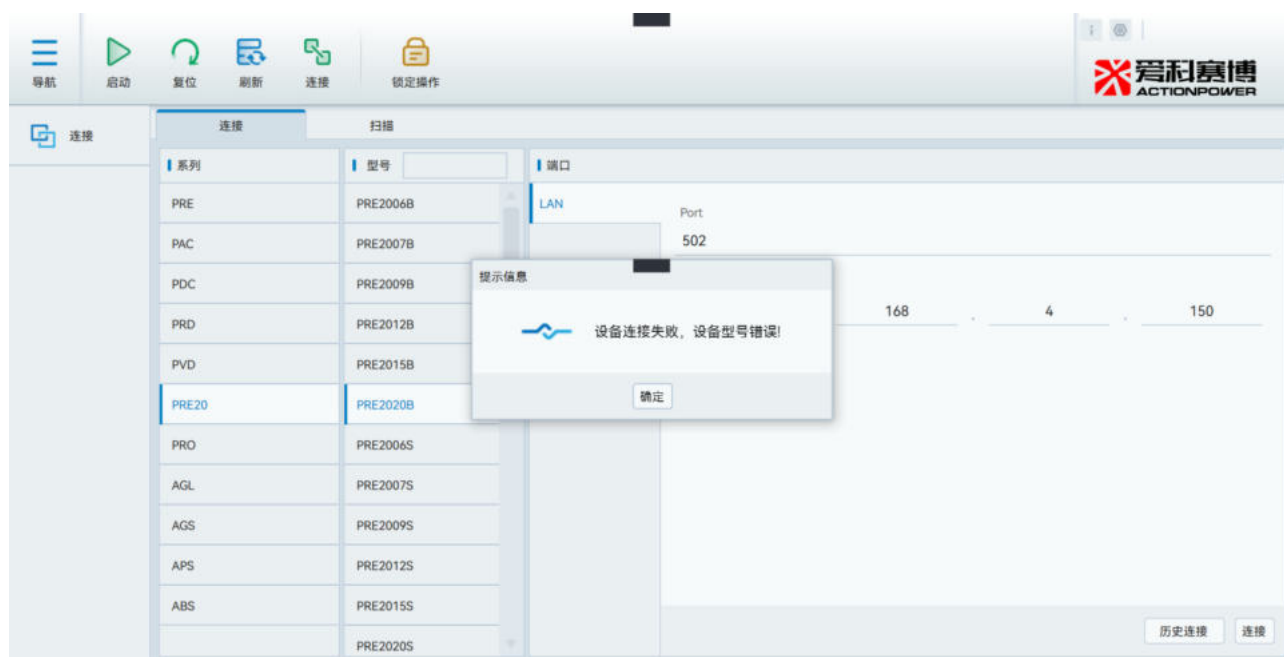
Figure 3.2.4 Connection Failure Due to Incorrect Model
