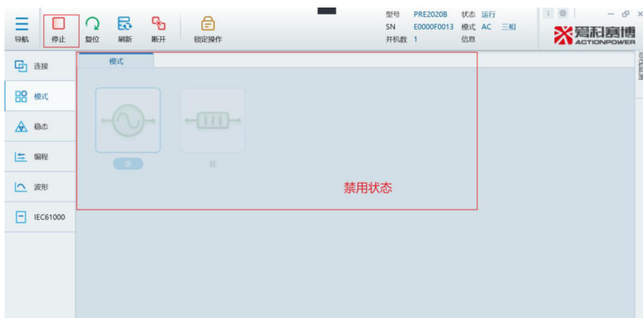
Figure 7.1.3 Mode Interface Disabled During Device Startup
