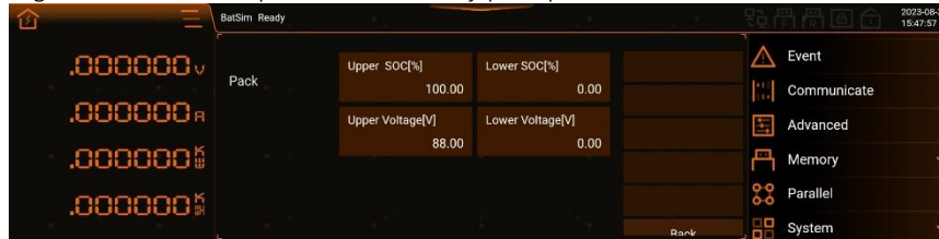
Figure 221 Battery Pack Protection Interface Figure
