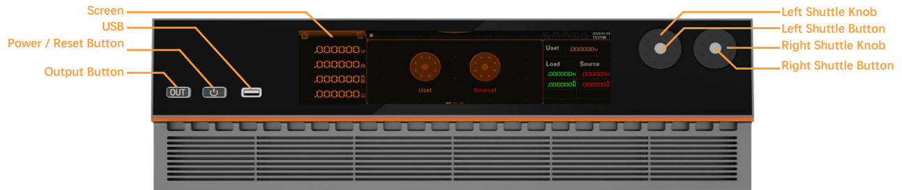
Figure 126 CD-B front panel functional partition figure
