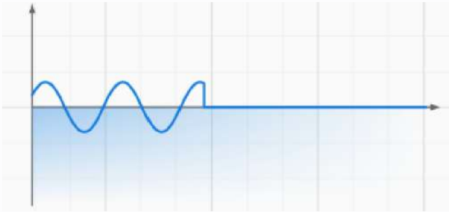
IEC61000-4-11 Interruption 90°@Class2/50Hz
